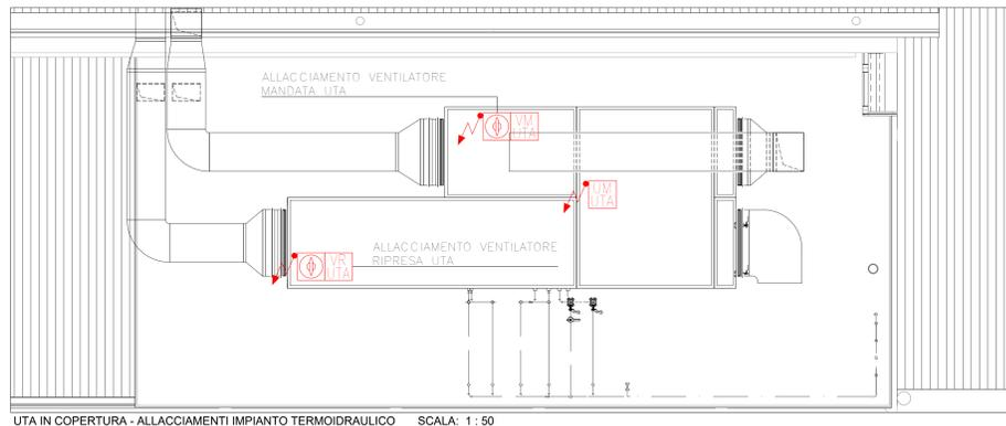
UTA IN COPERTURA - ALLACCIAMENTI IMPIANTO TERMOIDRAULICO SCALA: 1 : 50
